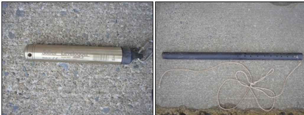
Figure 10 Solinst Model 3001 Levelogger Gold and still well. Photographs by N. Neatt, 2008.
